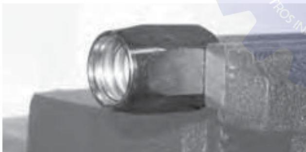
Socket positioned in vice.
