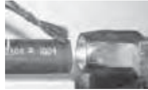
Apply lubricant to hose cover.
